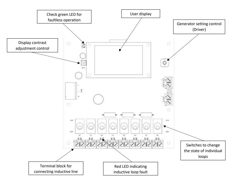
During normal operation, the generator display shows the generator firmware version and the vendor designation.
